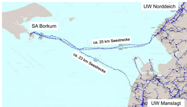
Figure 3 grid connection 20kV to the mainland
